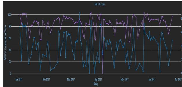
We reported the issue to vessel owners and in further investigation and communication with vessel crew we identified that error in the FO report was due to fuel flow meters. They rectified the calibration issue associated with the fuel flow meters and corrected the reporting.
